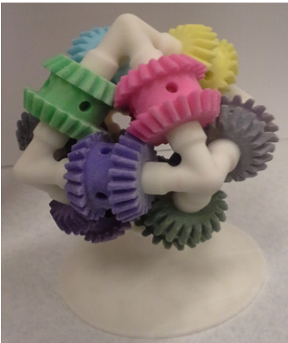
Keep interconnected parts moving parts to prevent the part from binding.
