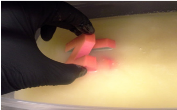
Dip part in wax. Use gloves or tongs if necessary.
