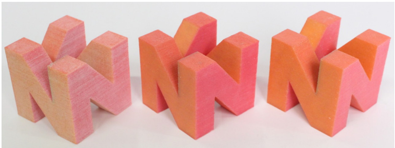
Left – Standard cleaning; Middle – IPA dipped; Right – Wax Dipped
