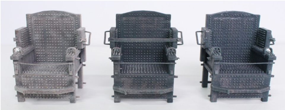
Left – Standard Cleaning; Middle – IPA 99% Dip; Right – Paraffin Wax Dip
