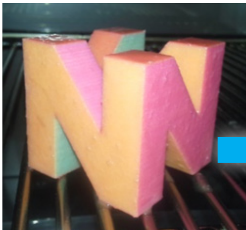
After dipping parts are covered in wax. Keep in oven to let excess wax drip off.
